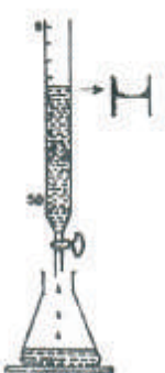
Fig. 15.1: Correct way to note down the burette readings
