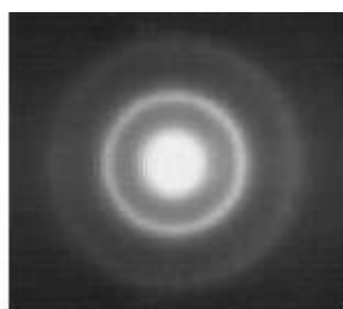
Fig. 2.13: Electron diffraction pattern from nickel crystal
