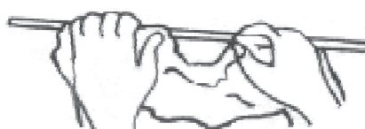
Fig. (ii): Holding & Breaking a glass tube
