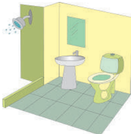
Fig.12.19: A water closet with a raised seat
